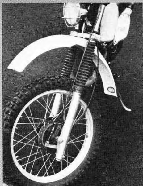
Forks from an RM-250C provide over nine inches of smooth travel. Air pressure can vary from 20 to 36 psi.
