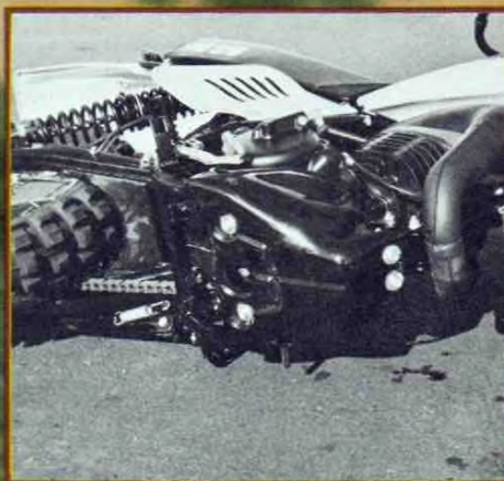
Steel skid plate protects well. Mounting bolts are recessed and trans oil may be changed without removal of plate. Kickstand spring is vulnerable to damage in rocky terrain.
