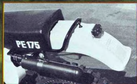
Spark arrester/silencer is quiet. Rear fender has flat spot on top for mounting a tool bag or carrying a spare tube.
