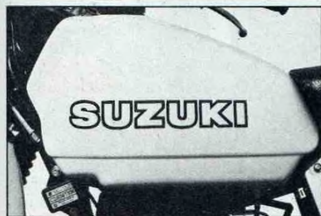
Large plastic gas tank carries the fuel low on the bike. Note staggered bottom.
