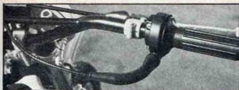
Throttle cable is routed back out of the way of tree limbs and brush.
