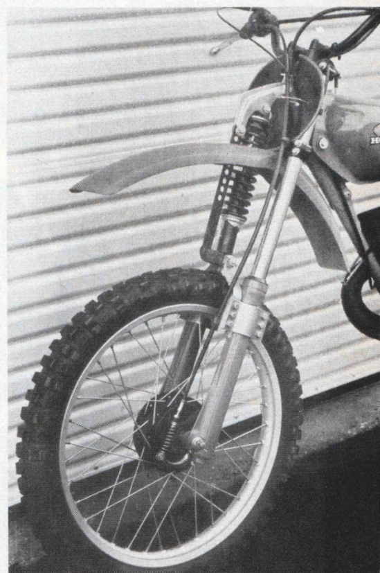
Axle should install easily if everything is right. If a good deal of pounding or tweaking is necessary to fit, then the clamps are off, loosen them and try again.
