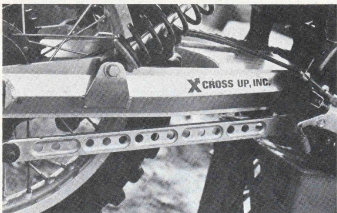
Swingarm is probably the strongest arm on the market today. Full floating brake unit pivots on heat treated axle.
