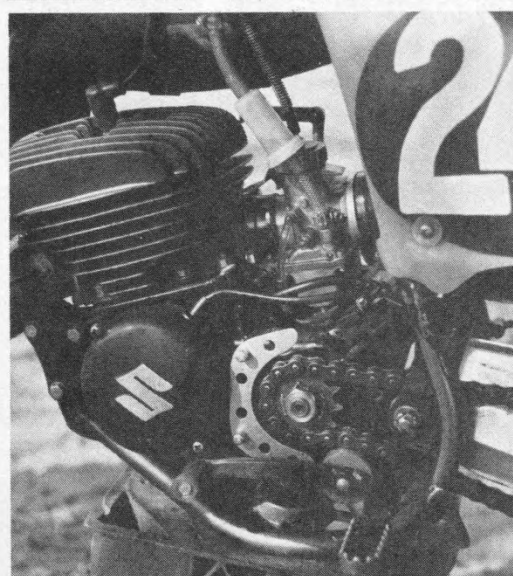
Carb is specially jetted and flow tested—works well.
