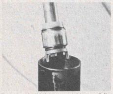
Remove shaft/piston assembly carefully, while pressing down on inner body. Hold inner body in place and drain oil. Clean all parts in solvent. Do not get any on O-ring or seal if you plan to re-use it.
