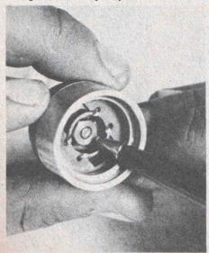
Check tension nut in foot valve. This must be tight, but must have small movement of flutter valve on opposite side.
