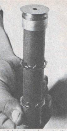
Install foot valve on inner vody. Place flat washer on top of foot valve while inner body is held upside down.
