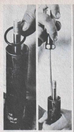
Install O-ring back in place. Press firmly in place with blunt instrument.
