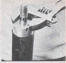
Tighten cap down. Stroke shock and if any air lock is felt, loosen cap and bleed air out.
