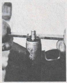
Using special tool, remove cap. Clean cap holes thoroughly before installing pins in spanner tool. Failure to do this could ruin cap.
