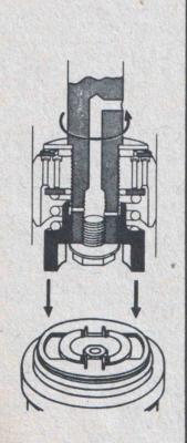
Fully collapse the shock absorber, at the same time turning the piston rod slowly to the left until it is felt that the teeth of the adjuster nut are engaging the recesses of the footvalve assembly.
