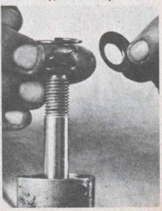
Remove spring and washer from shaft assembly.
