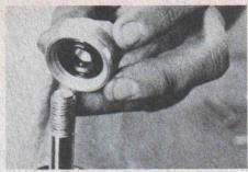
MODERN CYCLE recommends that you not use the stock Koni seal and cap because it's prone to leakage. We have used the Number One Products Koni cap with great success. The seal is part of the cap and of the spring loaded variety. Put tape over threads, grease lightly and slip the cap in place.
