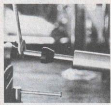
Place eye in vise and loosen jam nut with 19mm wrench. Remove eye and jam nut, then slide off rubber bumper.
