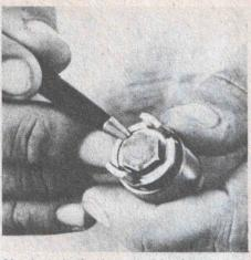
Check bolt in bottom of piston shaft assembly for tightness. Use an 11mm deep socket. This comes loose easily.
