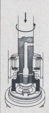
Continue to turn gently to the left until the rotation stops. Do not use force or attempt to turn further to the left, once resistance has been felt. At this point you are assured that shock absorber is in the unadjusted or new position.
