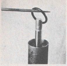
Using small screwdriver or pick, pry out O-ring, taking great care not to damage any more than necessary.
