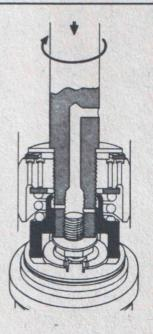
Now keeping the shock absorber collapsed, begin turning in the opposite direction, to the right. You will be able to make four half turns of 180° and a final quarter turn of approximately 90° to full hardness, each one of which is an adjustment compensating for approximately 20,000 miles of riding, depending upon the usage. You will know when you have reached the maximum adjusting position because you will encounter another stop. Do not force. will encounte Do not force.
