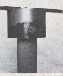
Remove spring from shock. Care should be taken in removing springs to not scratch the rod. If a screwdriver or any sharp object is used, keep it away from rod.
