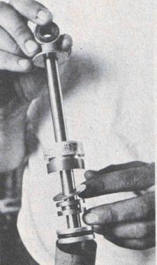
Withdraw rod, piston and seal retainer/ bearing, as a unit, from shock body. Care must be taken not to mar top surface of shock body, as this is a critical sealing surface.
