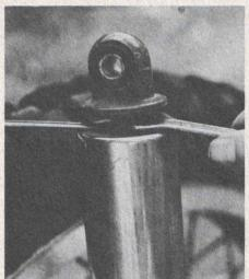
The top of the shock will now slide off and you can re-secure it in the bottom fork leg. Now use a screwdriver to move the dust cover down and slip a 17mm wrench onto the jam nut.
