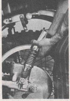
The dust cover slips under the 17mm nut and you can hold the shaft with a 10mm wrench.
