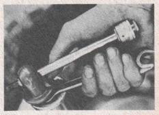
Run the top piece of the shock on with your fingers, then catch the 17mm nut. The old shock rod is a good tool for tightening. Replace all the mounting rubbers and bushings supplied in the kit and you've done it.
