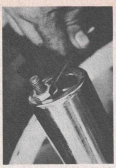
Run the 17mm jam nut on the shaft to the bottom of the threads, slide on the spring and dust cover.
