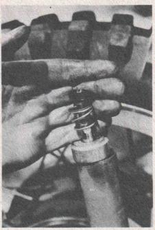
Slide in the new piston and rod assembly, then the upper cylinder block, rebound spring, tensioner cup, tensioner, spring (new), and seal (new).
