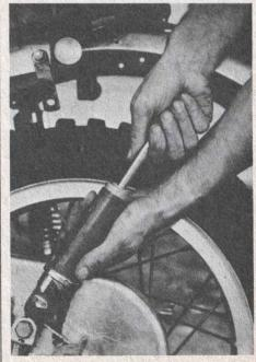
Hold the shock housing with one hand, grasp the rod with the other and remove the piston assembly.
