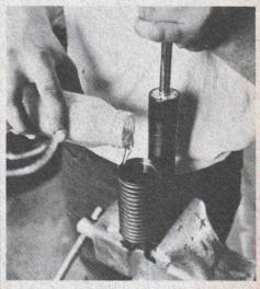
Add 175cc (6.0 oz.) shock fluid to reservoir. Install reservoir cap bolt. Torque to 175-200 in/lbs.
