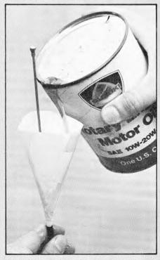
For the tried and true paper cone method, tape a cone of heavy paper around one end of the cable, fill it with oil and hang overnight. By morning you'll have a lubed cable, and a puddle on the floor.
