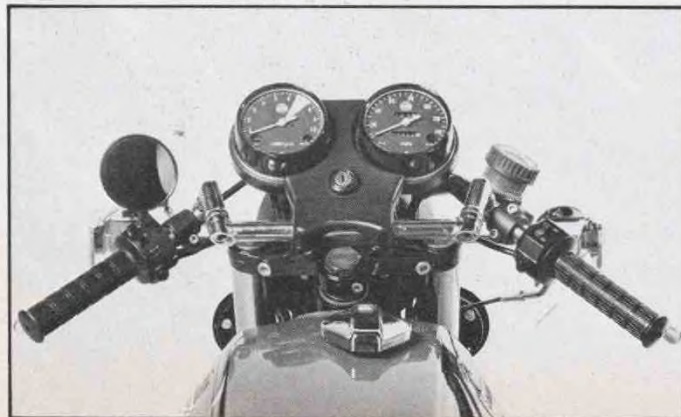
Adjustable handlebars are shown in the lower (cafe racer) position. They can be rotated-up into a low sport-bar position with the allen wrenches supplied in tool kit. Tool kit is second only to BMW's in quality.
