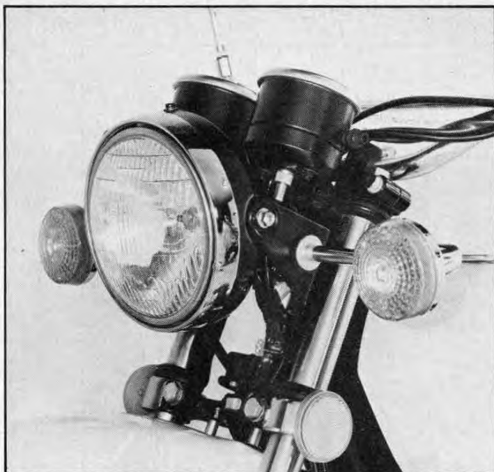
The entire headlight cluster, including tach and speedo, can be removed as a unit for serious off-roading, and to reduce weight.
