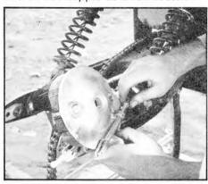
Stock brake shoes and cam mount directly on the new backing plateeverything fits perfectly.
