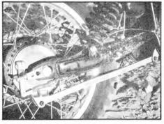
The full-floating Posi-Brake kit is similar to the Suzuki works-type brake and increases braking performance but requires a lot more attention. Pivot-arm angles and locations are critical to a full-floater's performance-MX Center did its homework.
