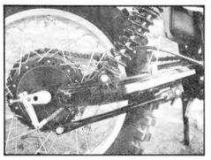
Most production MX'ers, like the RMs. use the conventional rear brake system utilizing the swing-arm-anchored torque rod. It requires no maintenance, but isn't as supple as a full-floater.
