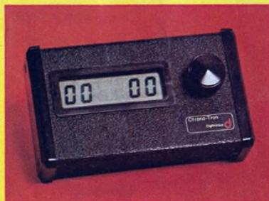
Digatronics' solid-state liquid-crystal enduro clock displays the time-of-day in minutes and seconds. Complete computers are also available.
