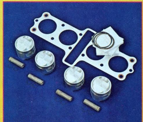
Yoshimura's 845cc kit for the GS750 Suzuki includes 69mm 10.5:1 pistons, pins, circlips, rings and a special head gasket. The \$140 kit was proven at Laguna Seca.
