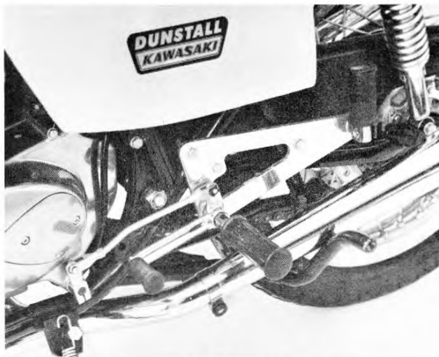
Craftmanship of rearset linkage is something to be proud of, retains down-for-low action. Good feel is retained without slop. Canted pipes clear curb.
