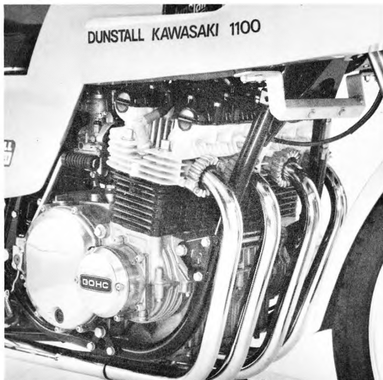
Dunstall 'glass fairing is secured in a very positive manner by this custom U-bracket to frame and again by a large U-bolt up front, around frame head. Test machine was Dunstall's own bike with beautifully finished 'glass work, but production model on a Mach III for sale at local Kawasaki dealership was dull and very unattractive. So quality varies.
