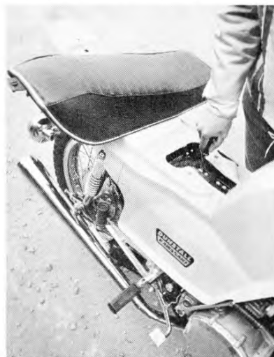
Dzus fastener secures saddle back, tongue and groove front. Brake leverage is insufficient.
