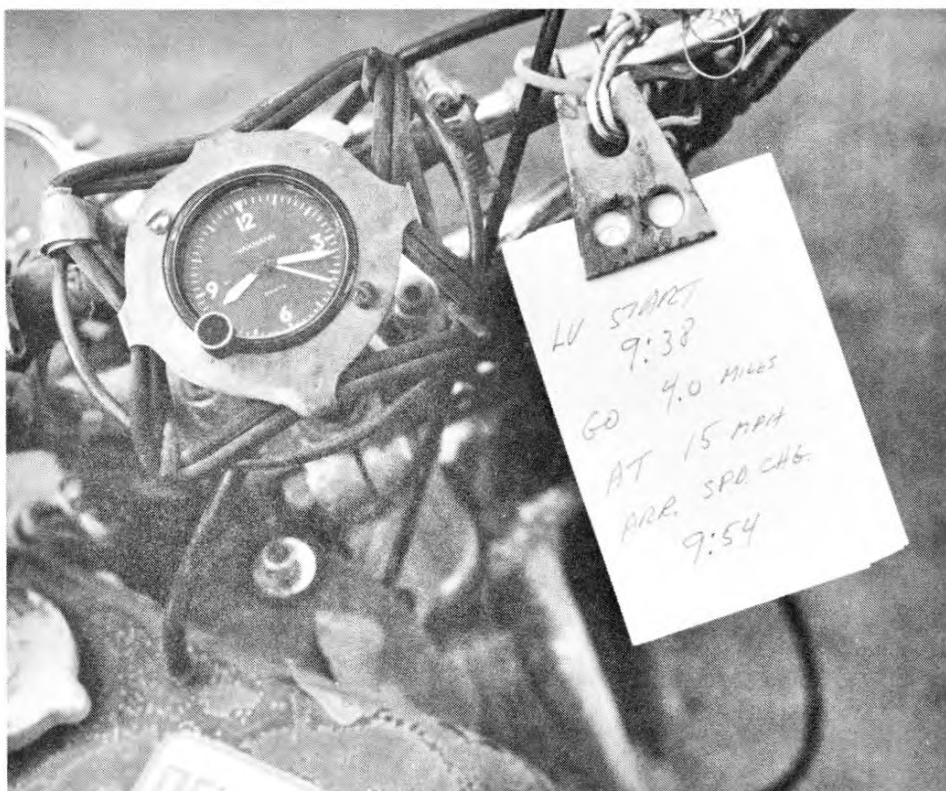
Enduro champion Bob Steffan's route information is nothing more than a stack of cards held with a heavy paper clip. Fine unless it rains. Clock is war surplus Wackmann model O-ring-mounted for shock-proofing during roller coaster ride.
