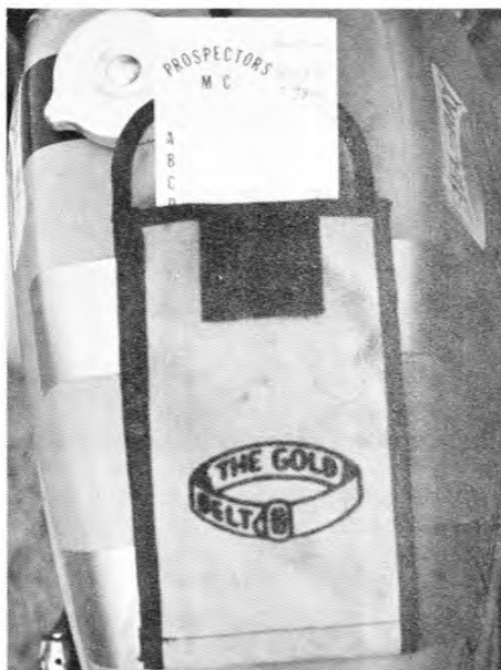
Do not fold, spindle, punch, lose or mutilate time card. Little Velcro closing pouch fastened to tank with silver tape secures and protects card.
