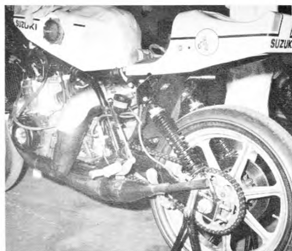
The mighty water-cooled Suzuki Triple that Lansivouri put on the front row of Yamaha Country. Long-travel suspension caused serious chain tension problems for team.
