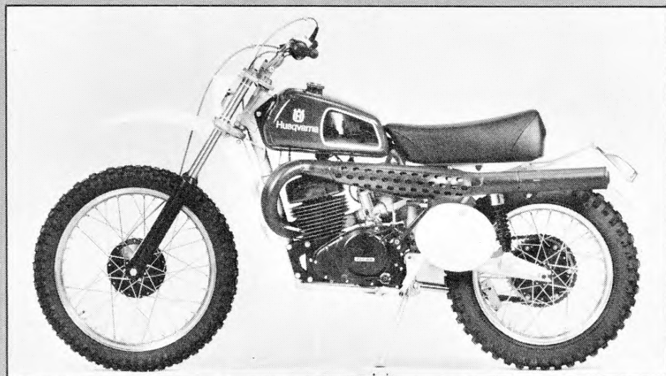
Preston Petty pieces are required to transform 400WR Husky into ISDT-type racer. Headlight/number plate was a snap to put on, Integrated Taillight/Fender took some fiddlin'.
