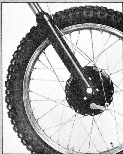
3.00/3.20x21-inch Barum tire is tad bigger than normal 3.00; we liked it.
