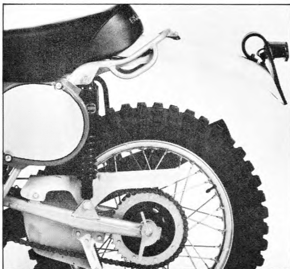
Telesco shocks are same as MXer's only fitted with lighter springs. Rear fender, chainguard self-destruct.
