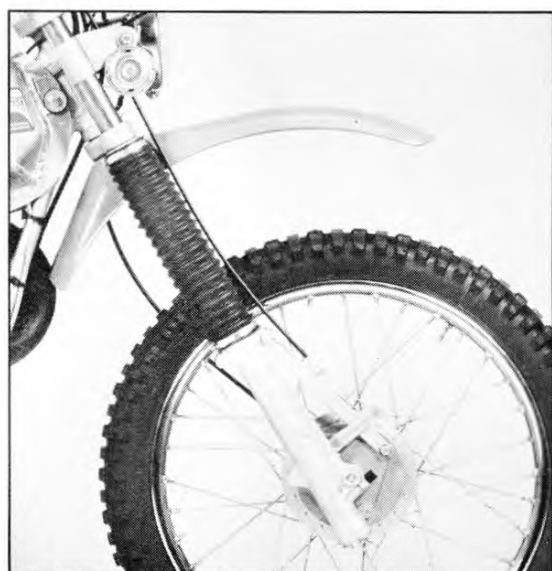
Headlight and horn turn high-pipe MXer into enduro mount. Tire rubs head pipe on compression, necessitates short fender.
