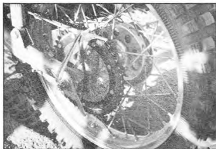
Left-side rear brake pedal is possible; wheel has been flipped over and sprocket repositioned.
