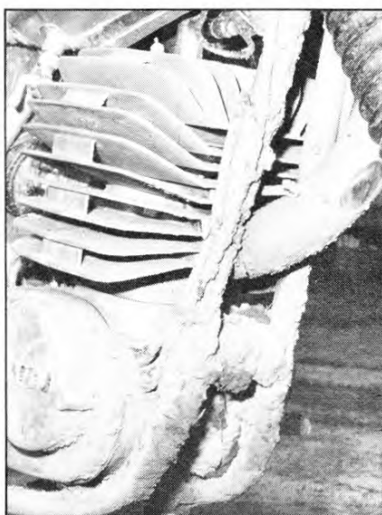
Clean cylinder fins offer little evidence of too-short front fender. Frame tubes got it.
