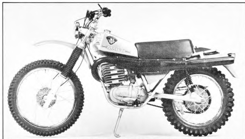
Center stand allows removal of either wheel without laying bike on its side. However, stand doesn't work on soft ground; bike just falls over. Lights and horn really work!
