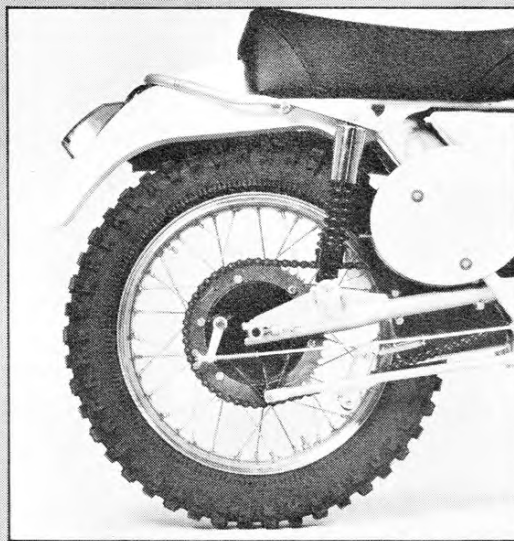
Girling shocks are almost mid-mounted, Husky claims 5.5 inches movement at rear axle.
