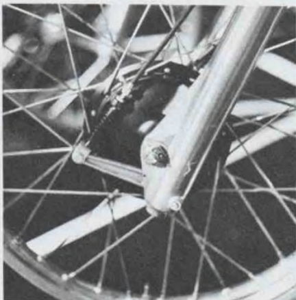
New leading axle forks are now featured on all three of the IT models.
