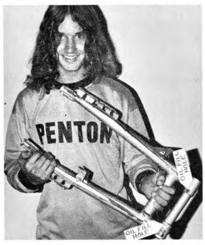
We took a trick right out of the Penton/ KTM book. Phast Patrick here holds a 250 KTM swingarm. You can see where the swingarm needle bearings are lubed by squirting oil in through two threaded oil filler holes, and when the swingarm axle housing gets full of oil, an appropriate bolt is screwed into each hole to seal it up . . . needless to say, you lube it with the swingarm still on the bike, nothing gets dismounted, just pull the bolts and add oil.
