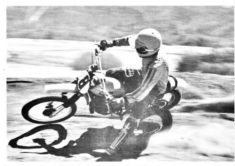
Shifting was somewhat stiff and the lever was too short to effectively shift the bike during competition. Using the clutch was a must when gas was on, as our bike refused to cooperate under power without a grab from the left lever every time you chose a new gear. A long lever would cure some of the shifting trouble, but owners will have to get used to using the clutch more often, in order to assure positive changes. Another of our complaints was about the choke lever.
