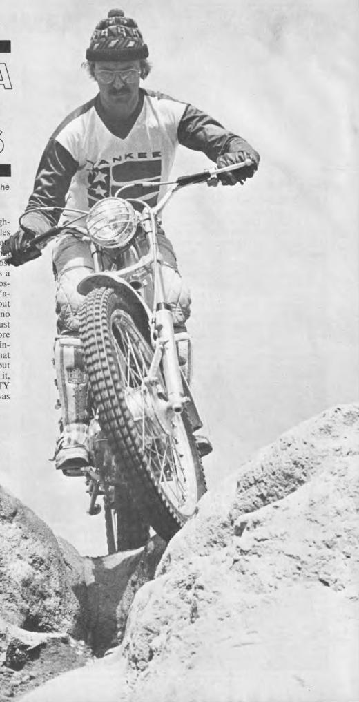
As delivered for test, our TY had the forks dropped in the clamps thusly. Steered reasonably well, quicker than the TY 250 tested last November.
