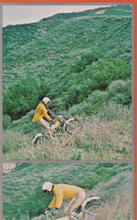
on smoothly which tends to turn sections into a series of leaps and lurches. Throttle turn is 90 degrees, which is about right, but if you remove the oil pump the return pressure is reduced enough to make control a little easier. Some additional flywheel and no more pump would make the 175 much easier to deal with.
