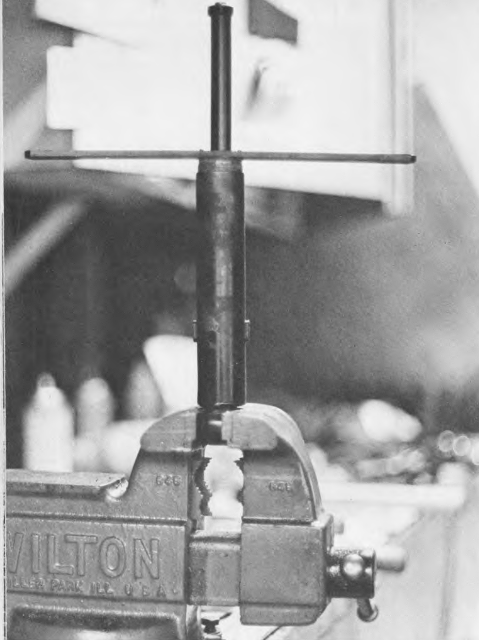
Koni tool gets strapped down by section of tubing and the nut that holds the cap on.
