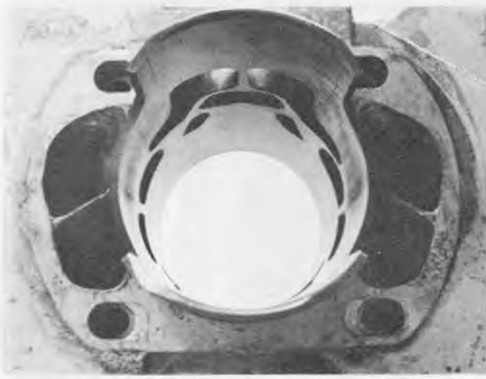
A manhole for a cylinder shows a lot of port area and few spots where rings always touch walls.
