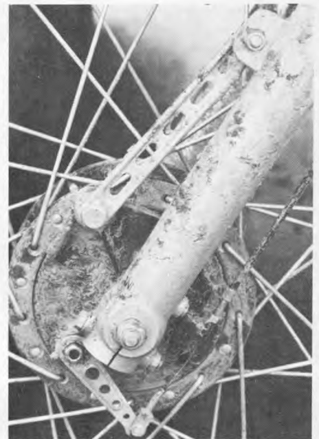
Forged aluminum torque arm and brake lever are improvements over stamped steel items of yore.
