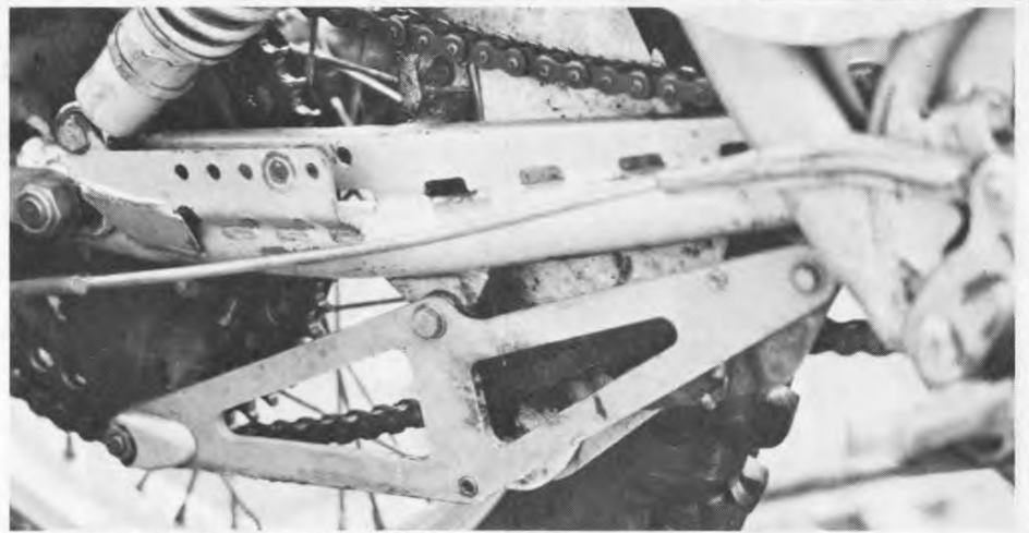
Cranke's own chain guard features a built-in chain tensioner, a must for cantilever suspension.
