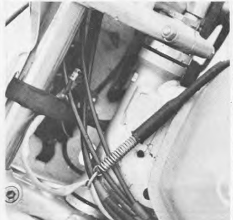
Double cables everywhere are routed for quick changes.
