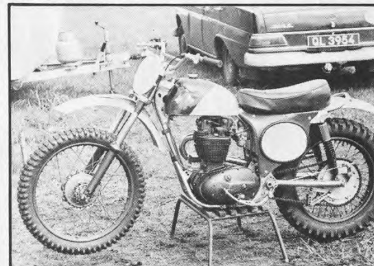
John Bank's 1970 factory BSA weighed 209 pounds and sported alloy seat pan, tank, airbox, number plates and fenders. Rims and engine cases: magnesium of course.
