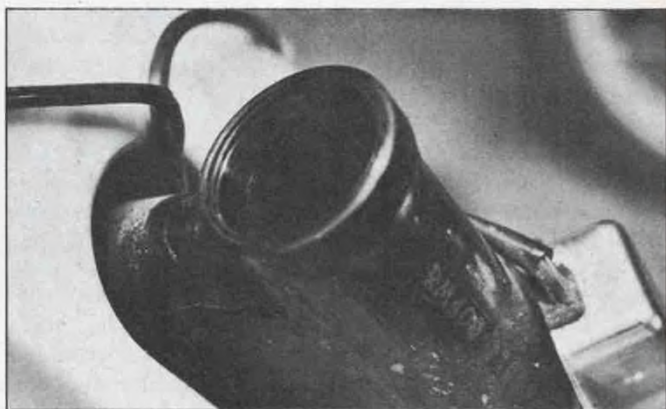
Tapered races tap into the head with no trouble.
