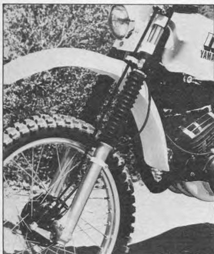
Spindly 32 mm forks have been replaced with heftier 35 mm units.
