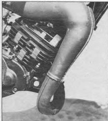
Lower edge of the pipe is vulnerable. Large belly is tucked in and will not make contact with riders leg.
