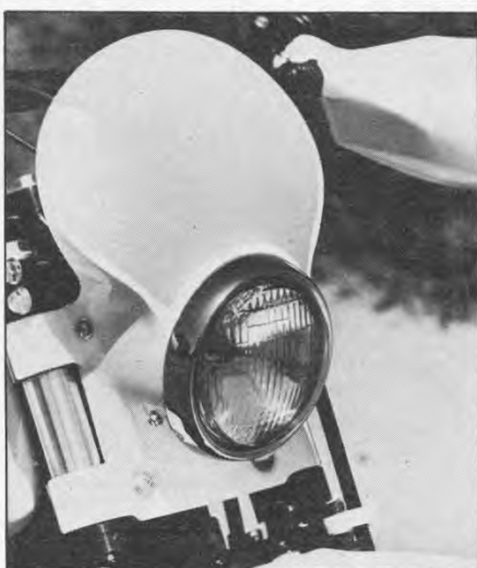
Combination head light/number plate is clean, but light shines mostly on the fender.
