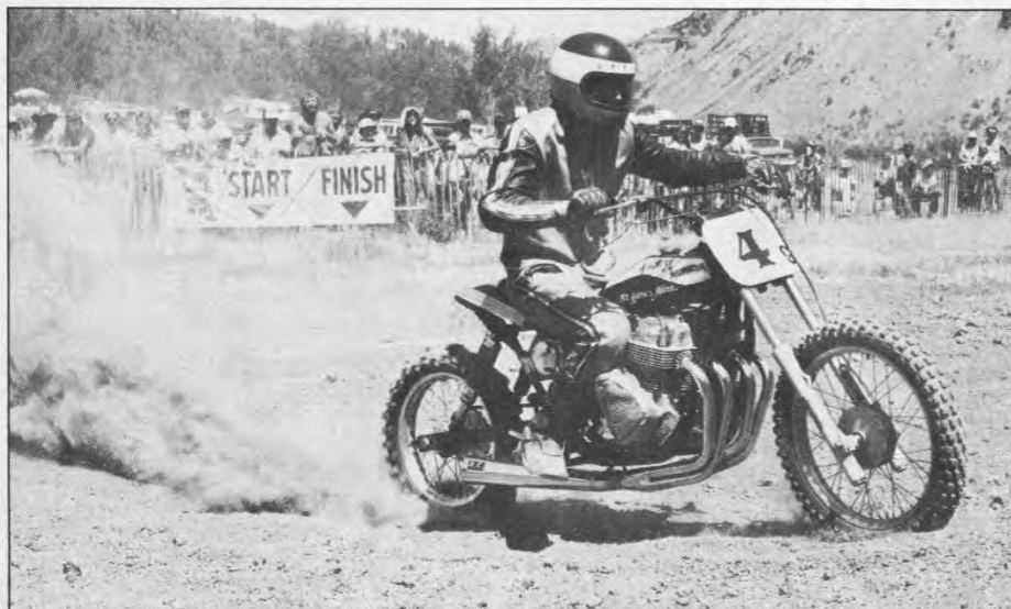
Some of the exotica came out in the Open class, like this four-cylinder Honda 750, with Simons forks and Fox Airshox.
