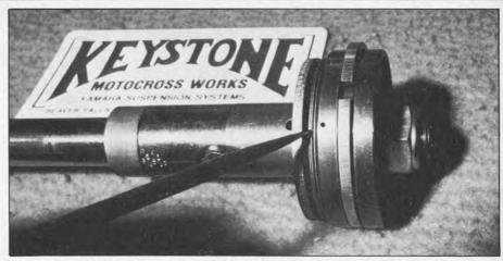
Here's what the new damping unit looks like fully rebuilt.
