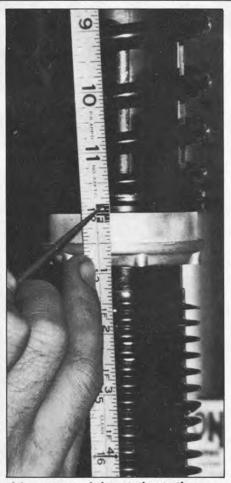
A large spacer is inserted onto the spring to compensate for the longer travel.
