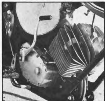
Pipe worked as the rear portion of droopy right footpeg, gas poured out around the cap, and the rear brake stuck.
