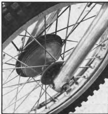
Check out that lightweight conical hub. The brake was for real.
