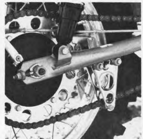
Swingarm on the D.P. is chrome moly rather than aluminum.
