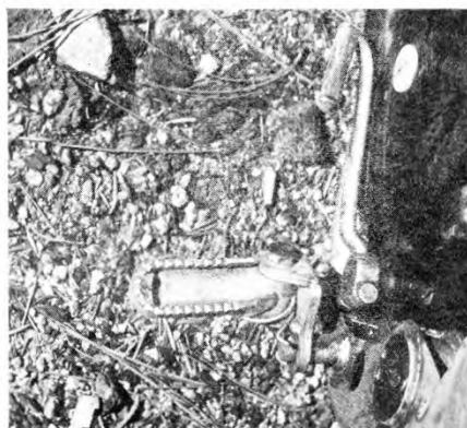
Both shift lever and footpeg took lots of abuse because of the Herc's lack of ground clearance. Folding shifter, please.
