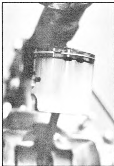
Two holes are added to the rear of the piston to line up with the third transfers which were lowered several millimeters, giving added scavenging from the bottom end.
