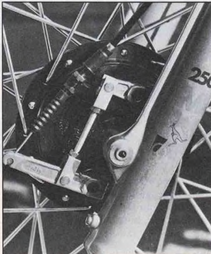
Both hubs share the same double-leading shoe setup.
