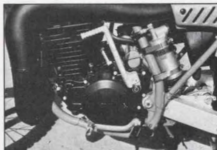
Now a five-speed, the Honda is versatile because of the torque motor and the new gearbox. The shock features both adjustable compression and rebound damping.
