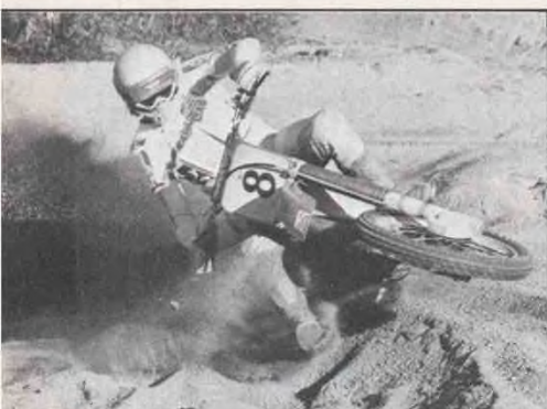
A sharp rake (26 degrees) makes for a quick handler. Slamming into a berm at speed requires a properly timed blast of throttle to keep you from plowing under.
