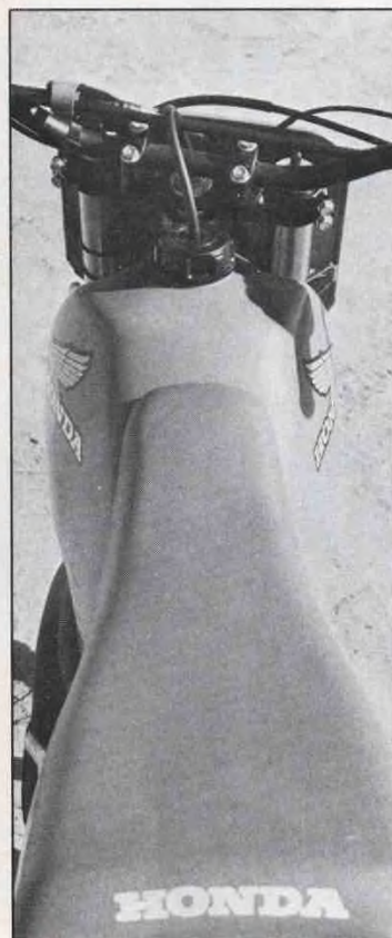
The tank is slim; this combined with the seat made for easy rider transitions. Shifting your weight around is smooth and natural.
