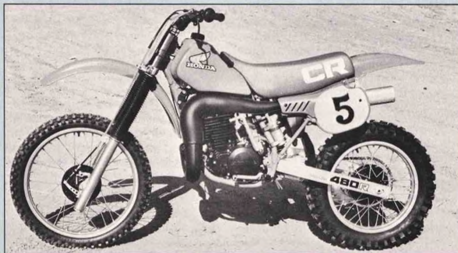
Although stylish and clean looking, the fenders allowed debris to be flicked up on the bike and rider. We eliminated part of the problem by installing a Gold Belt DeFender on the front.
