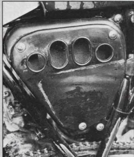
Some of the Kawasakis have rubber plugs on the airbox. On these models you don't have to drill—simply pop out the plugs.
