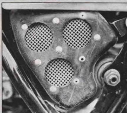
On '82 Yamahas, drilling the airbox is a must. The left side should have screen riveted behind it to keep garbage out.
