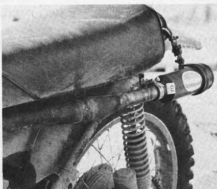
With the job done, the new pipe still fits in the same space as the stocker.
