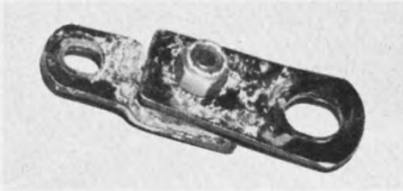
Hot setup for those rubber-cushioned brackets is to drill them through and use a bolt. Just tighten enough that the locknut won't loosen and it'll still cushion, without going south.
