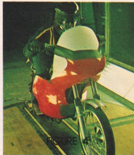
Two touring adaptations of a racing fairing: fuel economy would improve 12.4-percent with the taller; nearly twice that in the configuration shown below.
