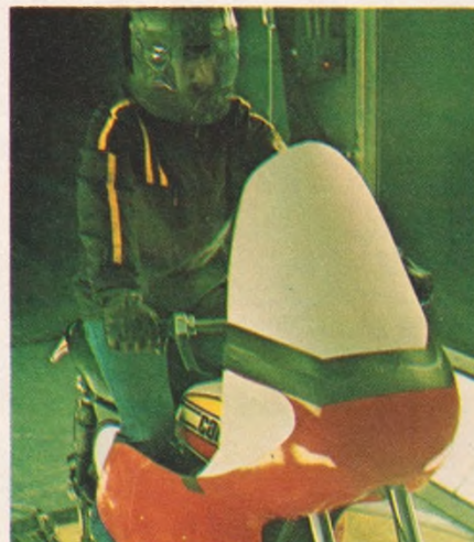
Two touring adaptations of a racing fairing: fuel economy would improve 12.4-percent with the taller; nearly twice that in the configuration shown below.
