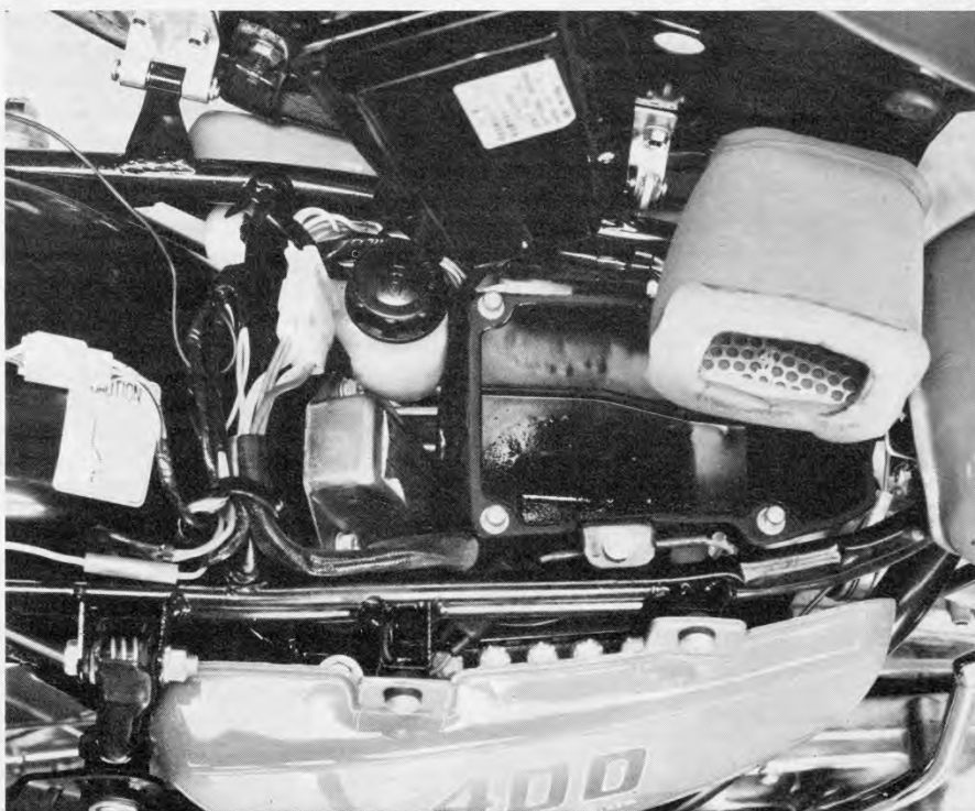
Under the saddle is a maze of paraphrenalia: wires, plugs, air cleaner, oil tank, and magic box.
