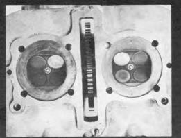
Pistons' view of four-valve heads. Intakes are 23.6mm in diameter while exhausts are 22mm across.
