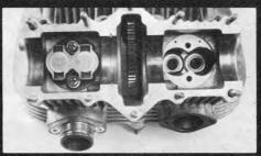
On left two tappets are installed in the guide block. With block removed, valve spring cavity is exposed.
