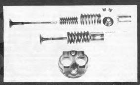
Upper tier: valve, inner/outer springs, retainer, keepers and tappet. Middle: nested assembly. Lower: block minus tappets.
