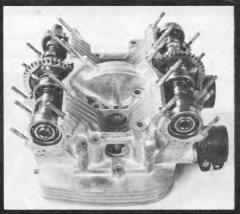
Engine had each camshaft running on four ball bearings. Spur gears drove the two overhead camshafts.
