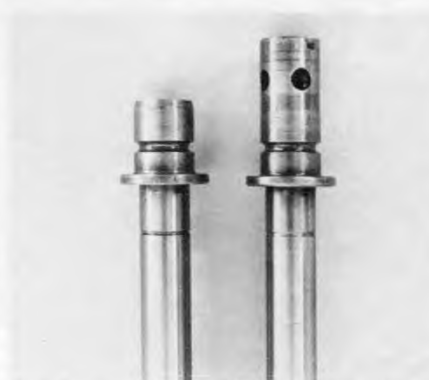
Can-Am piston rod (right) directs oil onto side of stanchion rather than up and onto fork springs.
