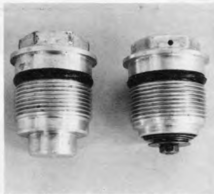
Can-Am 250's top fork nut permits air to escape on compression so no hydraulic air lock can occur.
