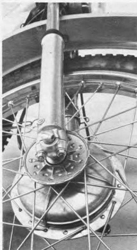
Conical style hub has a bigger brake and is too touchy. Fork action is good, springs bad.
