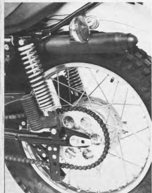
Shock springs are far too stiff; the brakes too grabby and the turn signals too vulnerable.
