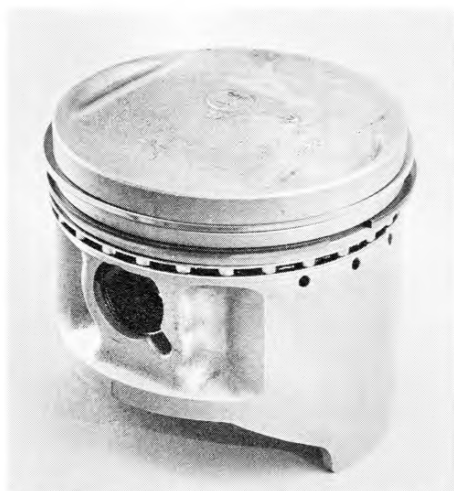
Cast aluminum piston is almost flat-topped, but has a slightly-raised area. Arrow points to exhaust pocket.
