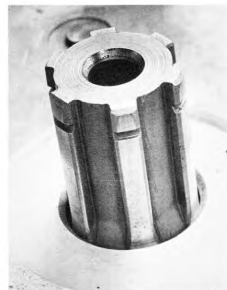
No nut secures the clutch to the transmission shaft. Instead a Seegar ring fits into this groove on shaft.
