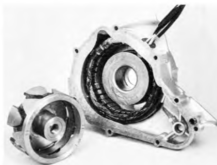
Standard-type alternator has inner and outer coils in left-side case; rotor spins on left end of crank.
