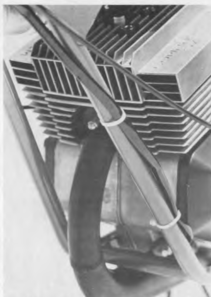
Ram-Air replica cylinder head finning does a good job of dissipating heat produced by the 3-cube engine.
