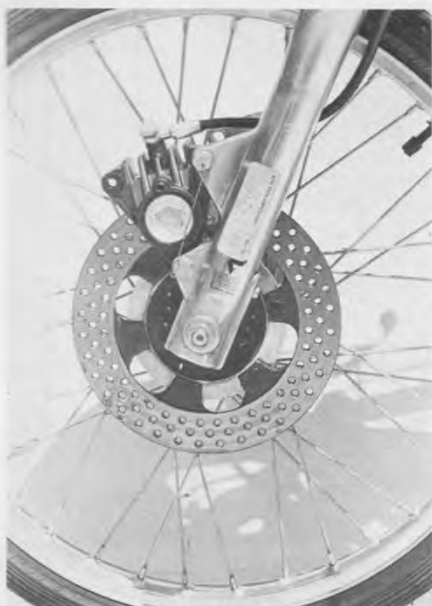
The horrific momentum of the blood-toned bullet is faithfully arrested by this tiny hydraulic disc brake.
