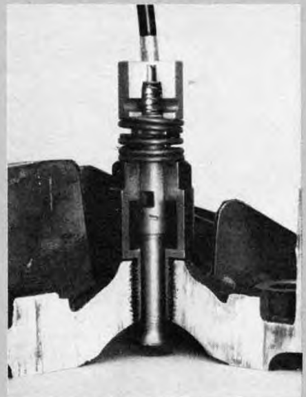
Fully opened, the ported valve vents combustion one-way to the atmosphere.
