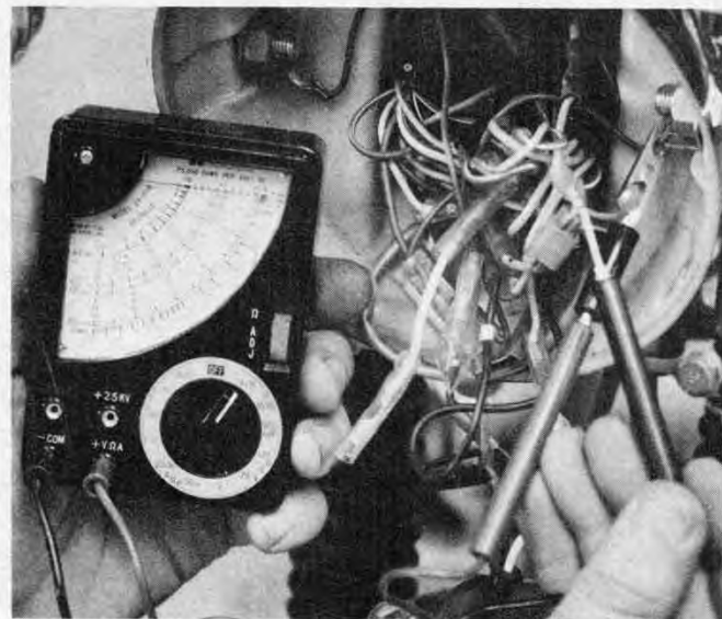
After disconnecting the yellow wires in the headlight, a continuity check shows the handlebar switch to be okay. A short in the harness!
