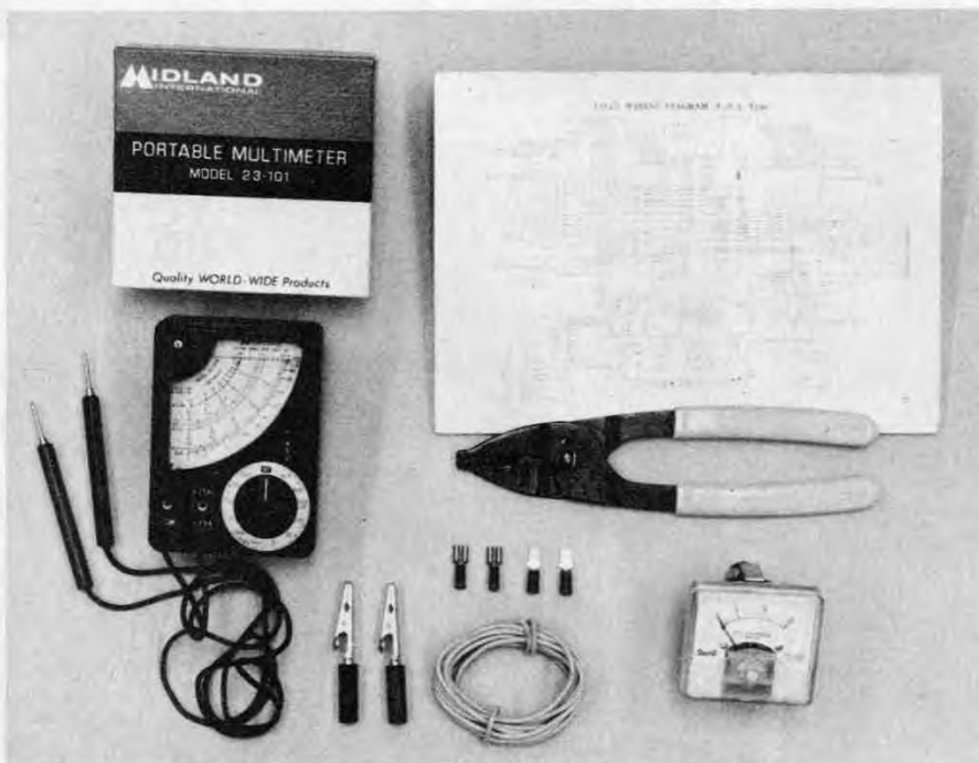
A cheap multimeter and a direct current ammeter are the basic tools for bike electrical problems. The wiring diagram, crimping tool, extra wire, and ends will make the job easier and faster.
