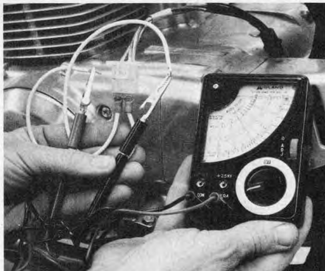
The first test is to measure the alternating current voltage at the engine. Measurement may be made with engine running or at kick-over.
