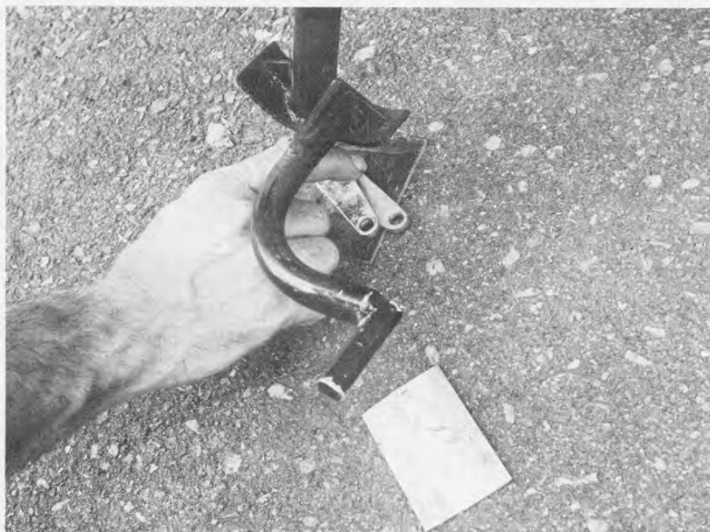
Getting proper vertical alignment (above; opp. page, below left) requires plumbob and string. Spacers under centerstand leg will be needed to get rear wheel vertical.
