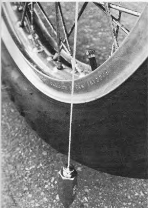
With front-to-back alignment straight, and the rear wheel vertical, the front wheel should be vertical too.
