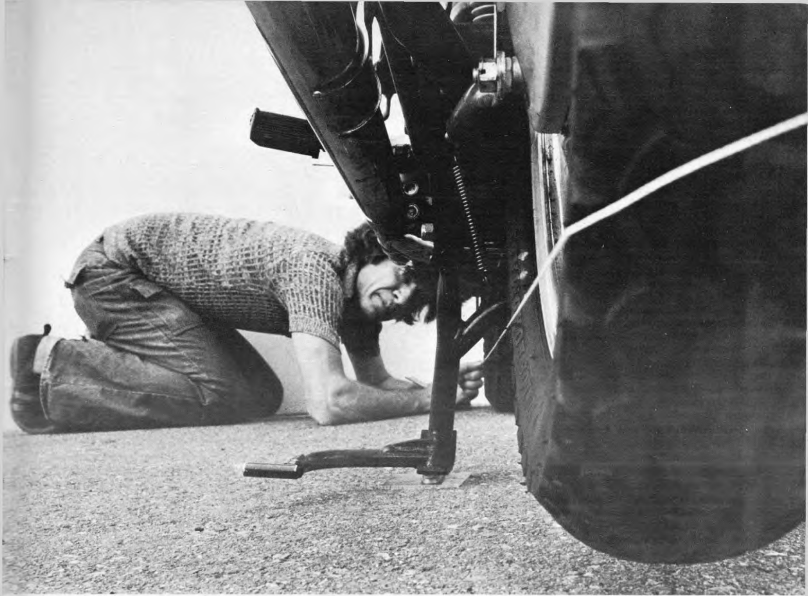
Front-to-back alignment can be checked with string and rule (above; center and right below). You may have to maneuver a bit to clear stands on some bikes.
