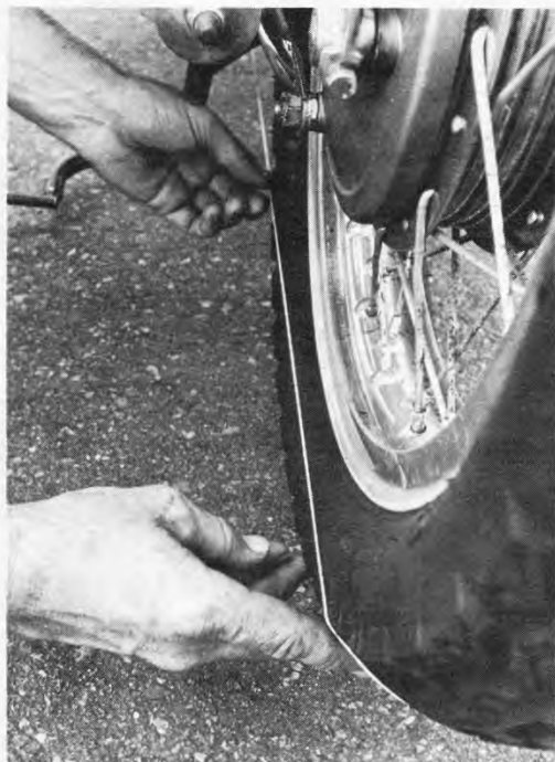
Be sure that you get a straight draw on the string which should just touch the rear tire's leading edge.
