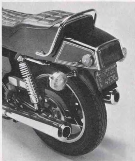
You can adjust the Suzuki's rear shocks for twenty different combinations of damping and preload.
