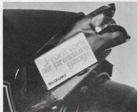
With this air pressure gauge, and a lot of luck, the GS1000's fork stiffness can be adjusted just right.
