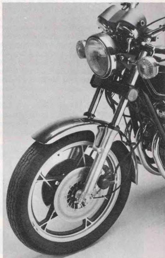
The dual-disc front brake is powerful, but puts a lot of weight where it isn't needed. Wheel doesn't help either.
