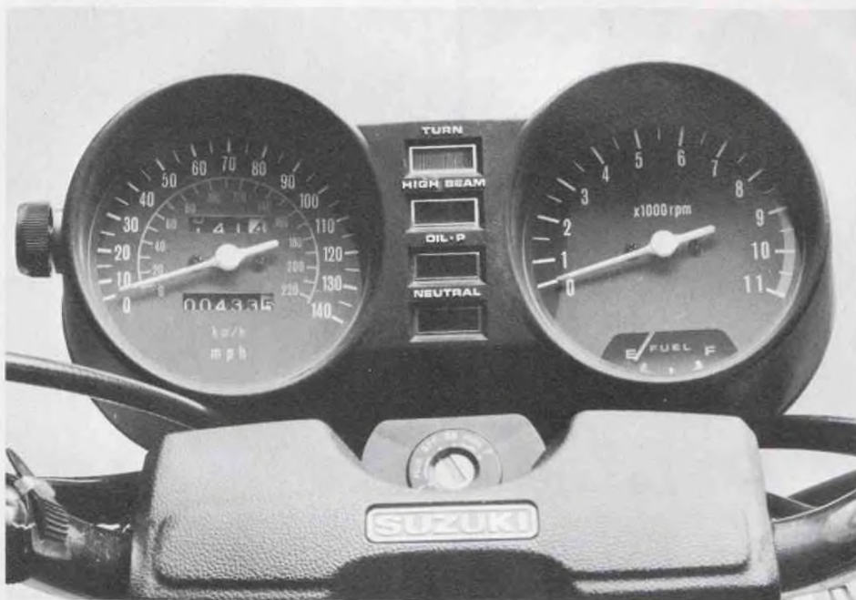
These poorly-calibrated instruments overstated speed, and underestimated the amount of gas left in the tank.
