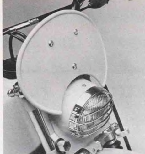
Guard protects headlight. Combination tool includes 13/16-inch plug wrench, 12 and 24mm box sections.
