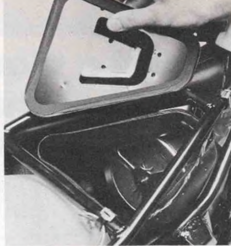
Air cleaner breathes through vented top cover, is waterproof—and mildly difficult to remove and service.
