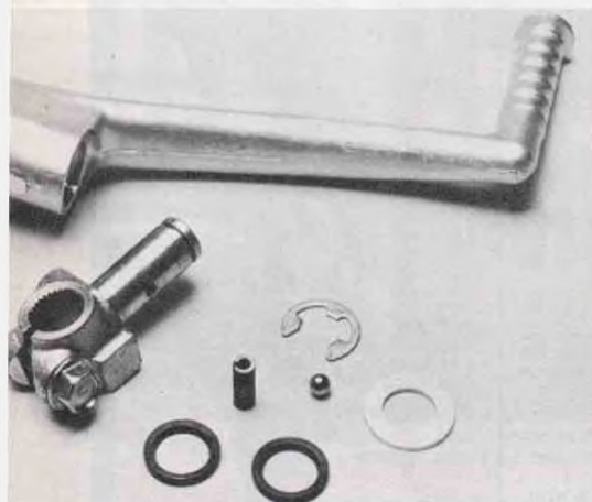
Miniature rubber seals are employed to keep debris out of the alloy-and-steel kickstart arm pivot...
