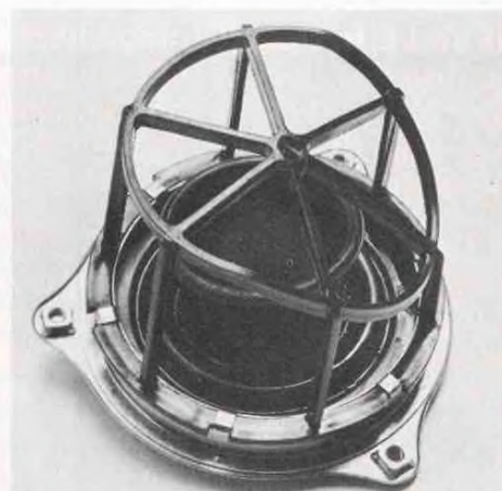
This dual-density foam filter (left) wraps around a metal and plastic frame (above) which contains a tuned carburetor velocity stack. A cover shields the left airbox side, and air is drawn in through the top.
